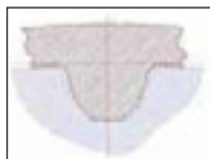
Eliminator tooth in RPP® sprocket groove
